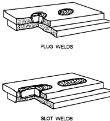
**Figure 3-18.** Plug and slot welds.
