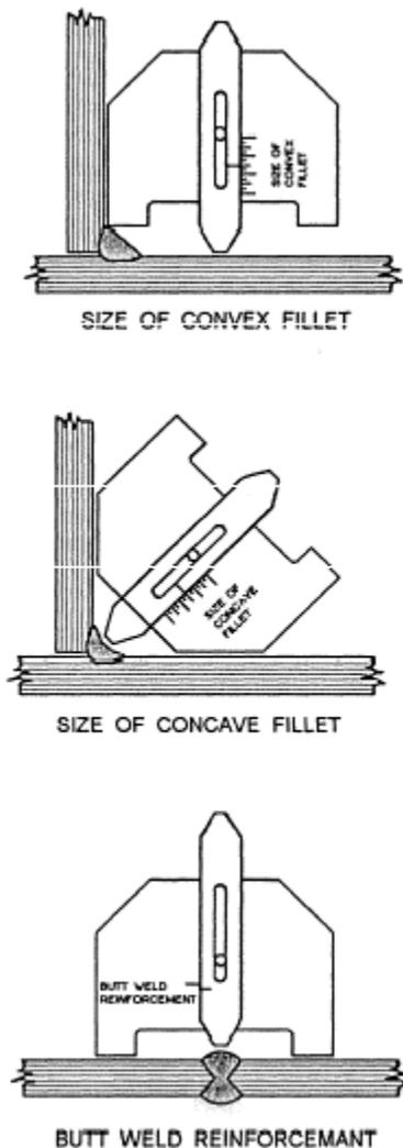
**Figure 3-21.** Using a welding micrometer.
