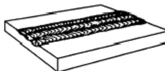
Figure 3-17. Surfacing welds.
