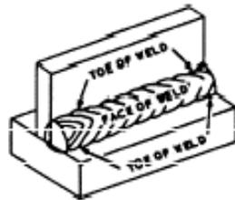
**Figure 3-20.**—Parts of a groove weld and fillet weld.
