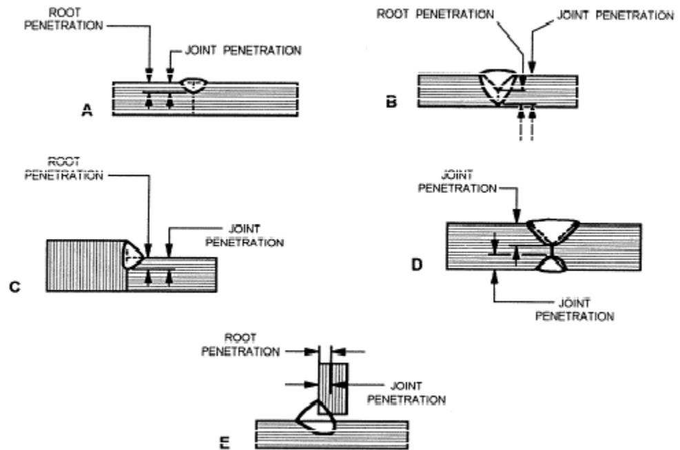
Figure 3-10.—Root penetration and joint penetration of welds.
