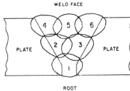
Figure 3-15. Weld layer sequence.
