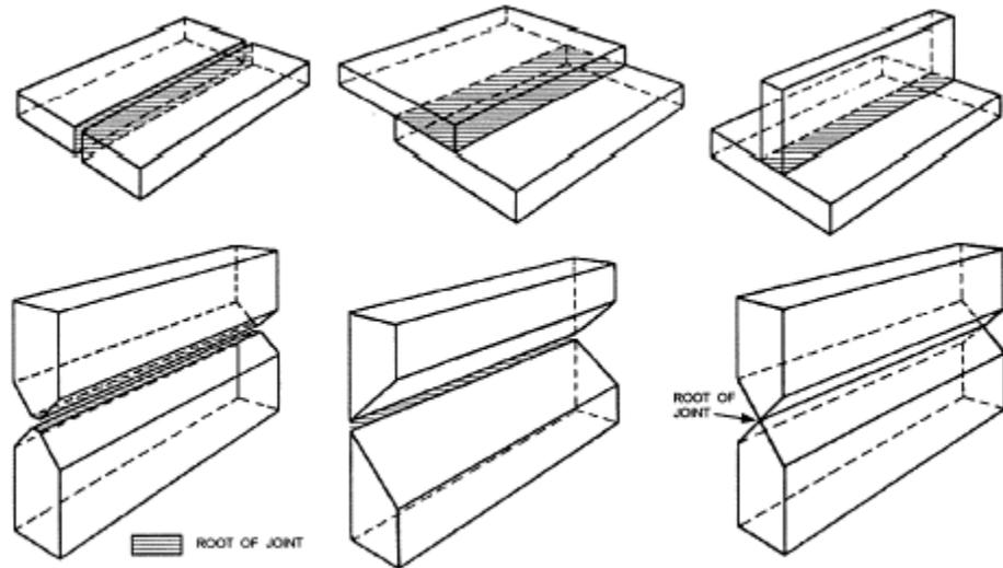
Figure 3-7.—Root of joint.
