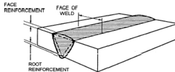
Figure 3-11.—Weld reinforcement.
