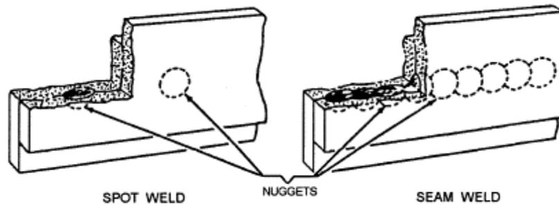
Figure 3-19. Spot and seam welds.
